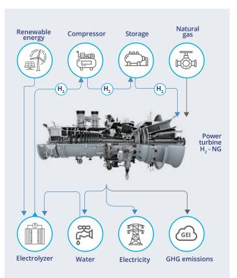
Hydrogen combustion is a very exothermic process that produces nitrogen oxides (NOx). To avoid emissions of this pollutant gas, turbine manufacturers are developing specialized burners that reduce the flame temperature. These burners are named Dry Low Emission or Dry Low NOx.
