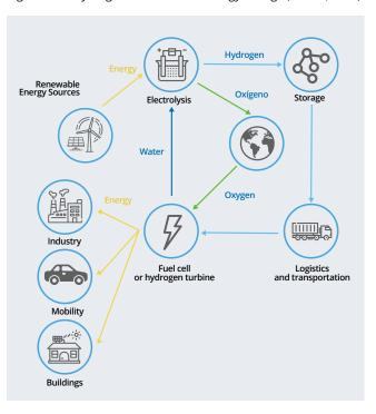
An electrolyser is an electrochemical device where water molecule is split into hydrogen and oxygen. Oxygen is vented and hydrogen stored on tanks or vessels. A fuel cell in a device with the opposite function, it is fed with hydrogen from tanks, takes oxygen from air and delivers electrical power and water. Alternatively and depending on the volume of hydrogen available, turbines can be used to convert hydrogen into electricity (see section 1.6).
