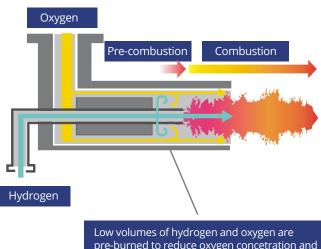
pre-burned to reduce oxygen and oxygen are then,flame temperature and its associated NOX emissions
