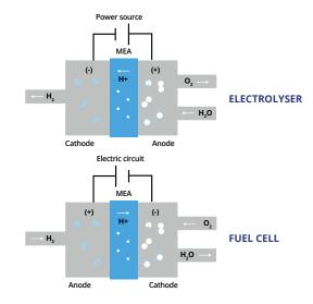
Fuel cells provide electricity to hydrogen vehicles (Fuel Cell Electric Vehicles). In stationary applications, they are used on power applications and low energy consuming systems from kilowatts to few megawatts (houses, telecom antennas, etc.). In high demandant energy applications and centralized power generation, hydrogen is used as a fuel for turbines of 20-400 MW.
